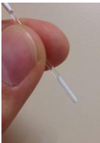
Figure 9. Photo of a pellet formed at the bottom of the capillary by centrifuging the lipid dispersion. Above the pellet is the phase-separated solution.
