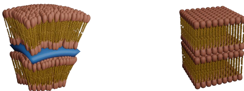
Figure 4. Left: Two stacked phospholipid membranes in a multi-lamellar vesicle. The membranes are curved bilayers with a water layer in-between, where the molecules are in liquid-like disorder in the plane of the membranes ( L_\alpha ). Right: Stacks of flat bilayers with long-range molecular spatial correlations composing the ordered crystalline ( L_c ) phase.
